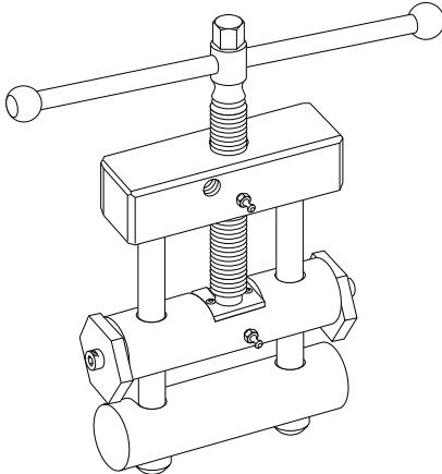
**Safety Considerations** — Pressure control situations requiring squeeze-off may involve working in the vicinity of escaping gas. Consider the possibility and potential hazard of static electricity and observe safety precautions. Precautions can be taken to dissipate the charge, and minimize the possibility of an ignition. This will maximize the personal safety of the crew. These precautions should be followed as a minimum, conditions may require additional measures.
